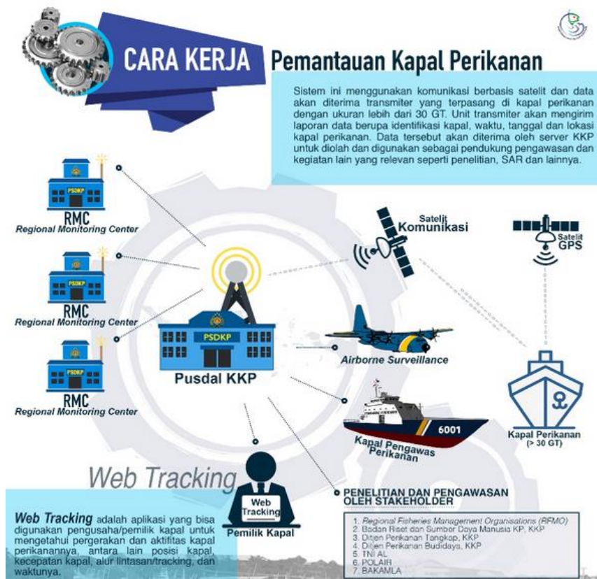
Gambar 13 Cara Kerja Vessel Monitoring System (VMS)
